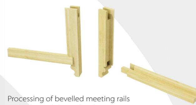
Processing of bevelled meeting rails and stiles with horn details
