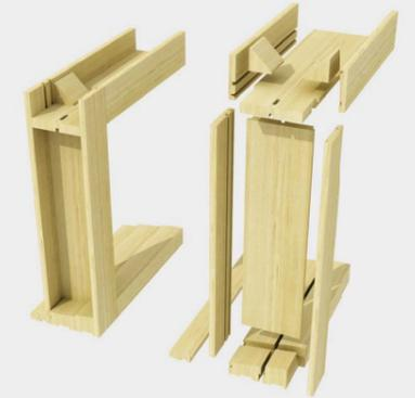
Trenching operations for pulley stiles and cutting of lining beads
