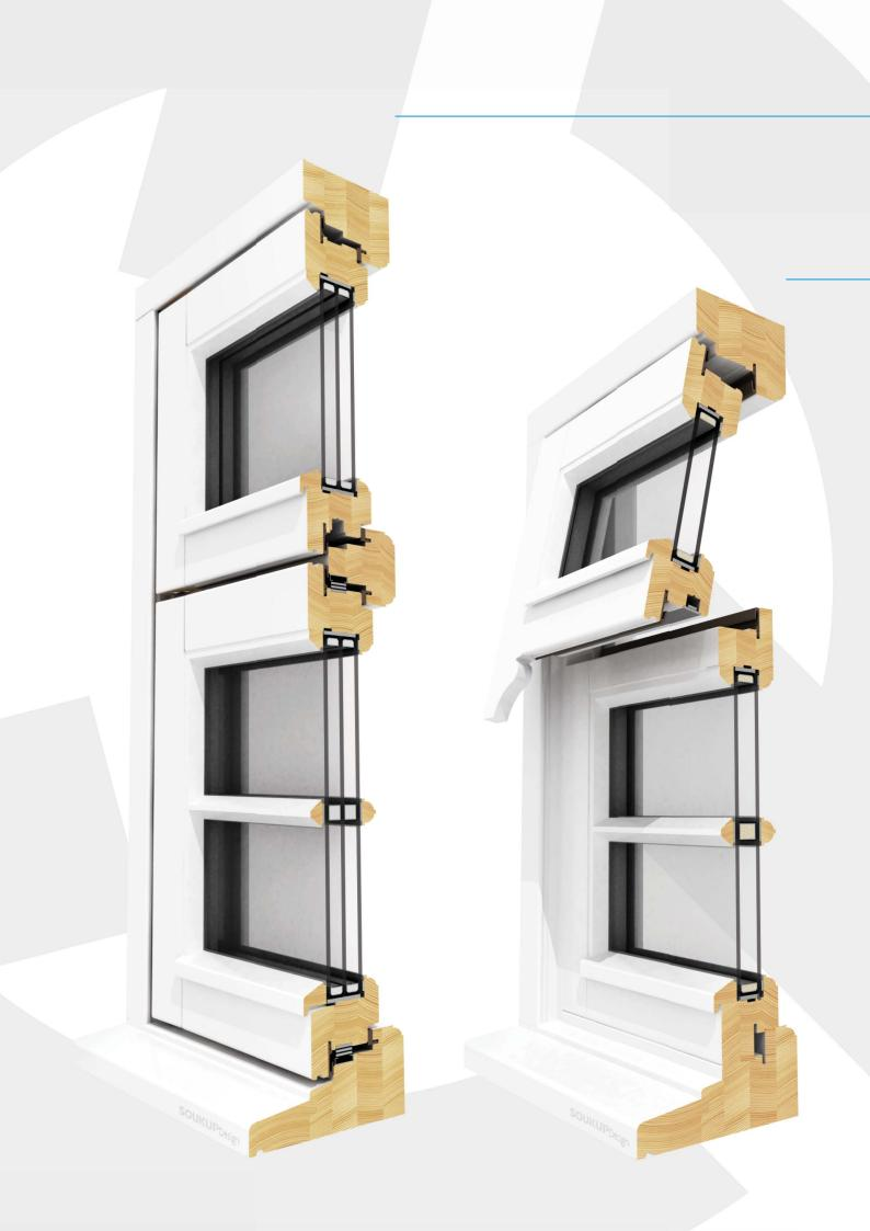
The High Performance Flush Window with a triple glazed unit meets the highest of requirements. The casement extension with a deeper glazing rebate for higher thermal efficiency does not disturb the flush exterior line. The projected glazing bead allows for required casement ventilation.
