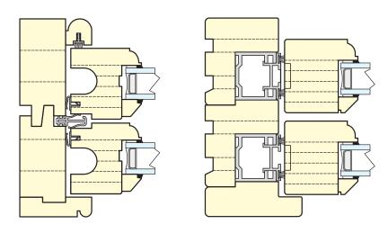
Traditionally manufactured box for sliding sashes balanced by lead weights. Industrial solution for sliding sash windows with spiral balances in a sash or in a box construction with a tilt mechanism. Individual design for parting beads, weather-seals or piles. Boxes consist of tenoned frames, fully machined on the window centre.
