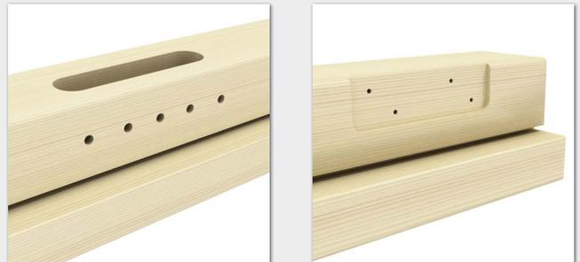
Longitudinal milling and drilling
