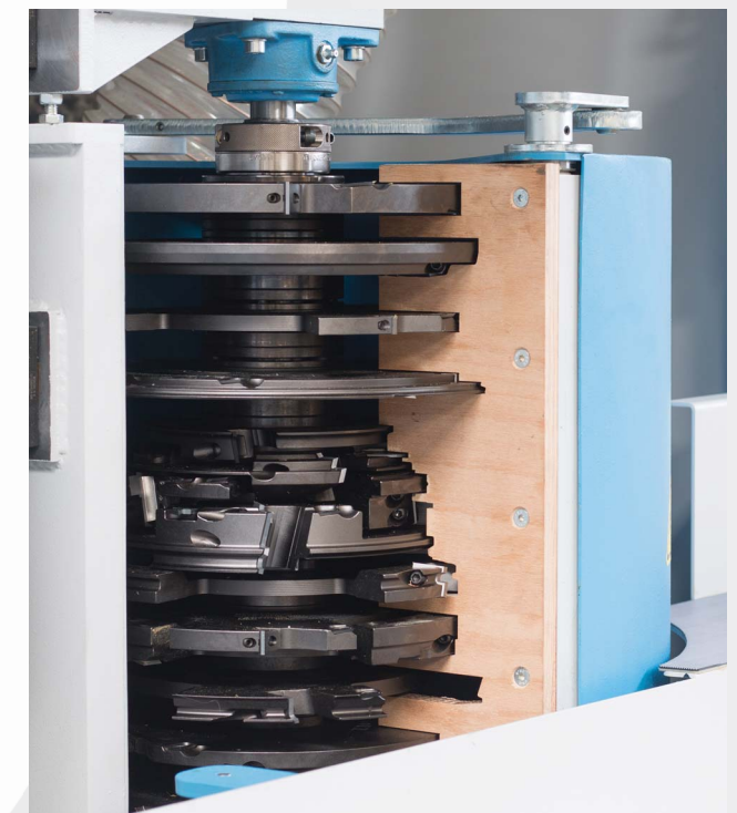
chip breaking device for tenoning matches the tooling stack
