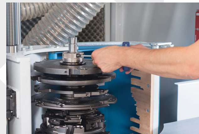
release hydro nut using allen key
