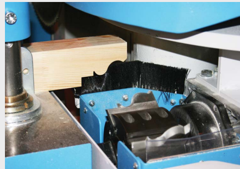
Horizontal milling unit for heritage sash horn detail or trenching of sash box (optional)
