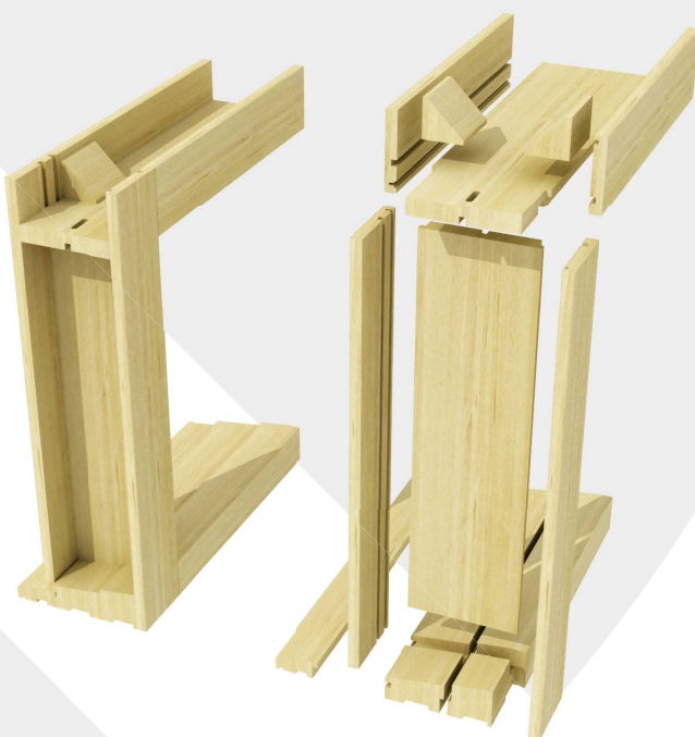
Sliding boxes made from profiled beads on the Crafter
