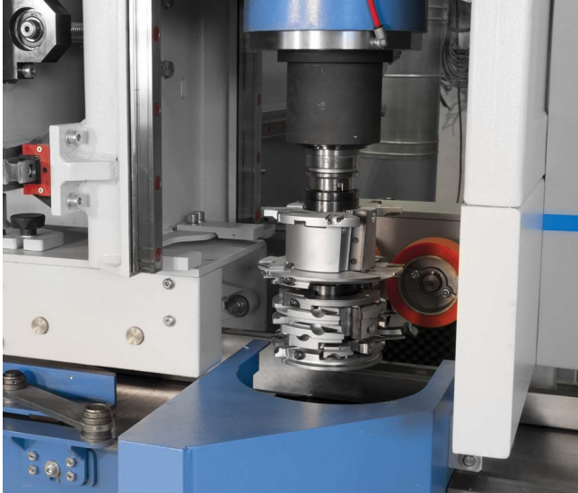
Profiling unit working from both sides
