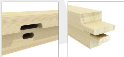
Mortised slots with rounded tenons
