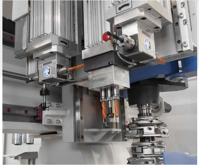
Tenoning spindle with drilling units
